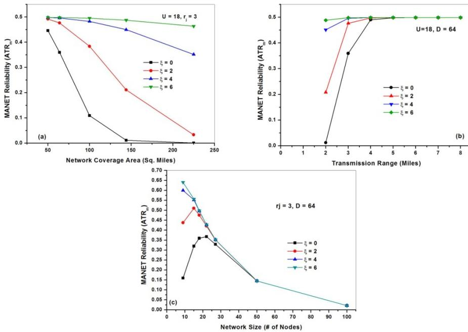
**Fig. 6:** Effect of (a) Network Coverage Area (b) Transmission Range (c) Network Size on ATR<sub>m</sub> for Different Values of  $\xi$ .
