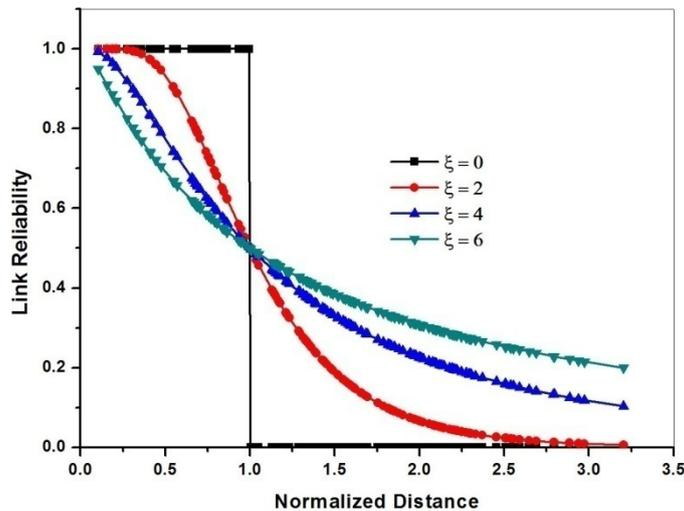
Fig. 1: Link Reliability as a Function of Normalized Distance for Different  $\xi$  Values.
