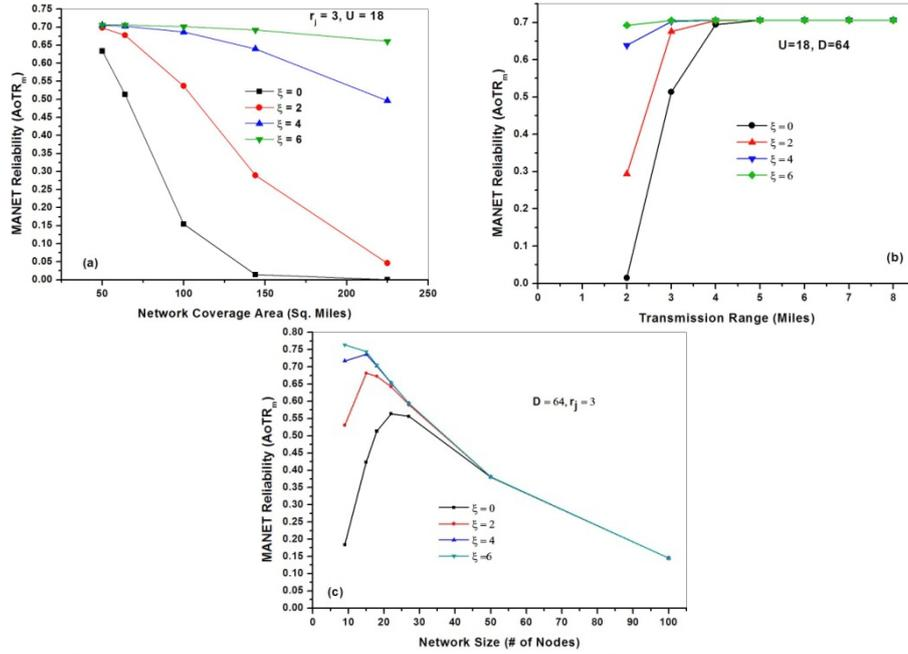
**Fig. 5:** Effect of (a) Network Coverage Area (b) Transmission Range (c) Network Size on AoTR<sub>m</sub> for Different Values of  $\xi$ .
