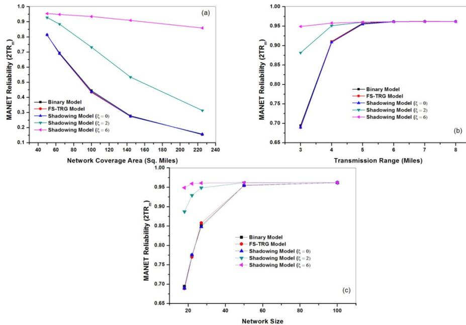
**Fig. 3:** Effect of (a) Network Coverage Area (b) Transmission Range (c) Network Size on  $2TR_m$  for different Link Probability Models (Binary model, FS-TRG model, Shadowing Model).
