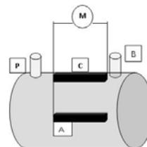
**Figure 3:** Solid MFC fed with Organic Fraction of Solid Municipal Wastes. A: anode; C: cathode; P: pHmeter probe; B: biogas sampling opening; M: digital multimeter.[35].
