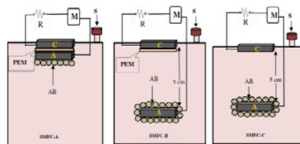
**Figure 2:** Schematic details of various configurations of Solid MFC used in [8] [A: anode; C: cathode; PEM: proton exchange membrane; AB: anodophilic bacteria; M: multi meters (digital display); R: resistance (100  $\Omega$ ), S: sampling port [8].
