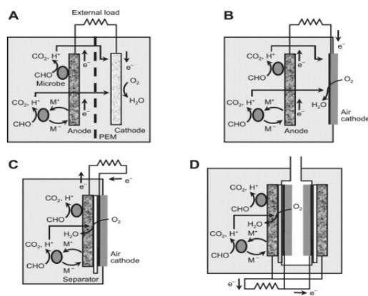
**Figure 1:** MFC configurations and electrochemical reactions. (A) A double-chamber MFC using oxygen as the cathode electron acceptor. (B) A single-chamber air-cathode MFC. (C) A single-chamber air cathode MFC with cloth electrode assembly separator. (D) A cassette-electrode MFC. M, Mediator; CHO, organics; PEM, proton exchange membrane. [20].
