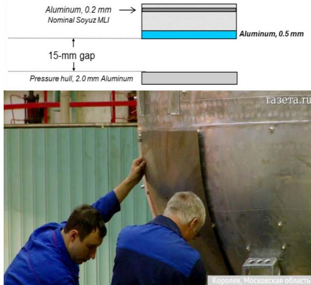
**Figure 6:** Improved Soyuz MMOD Shielding
