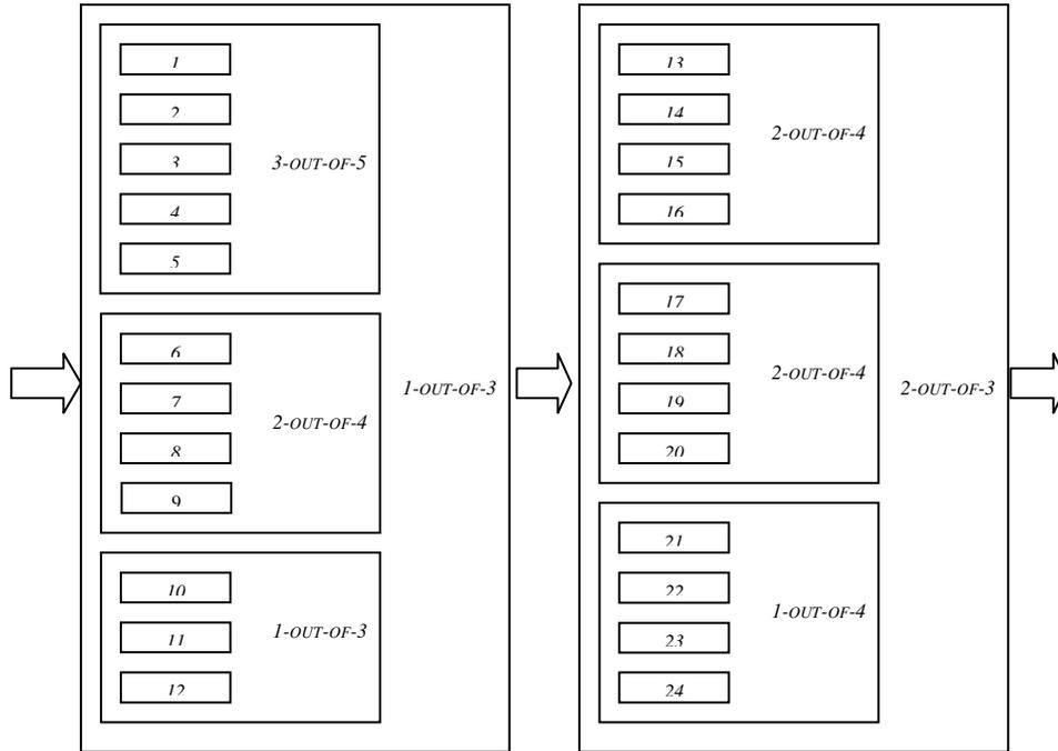
**Fig. 1: Configuration of RAID System**
