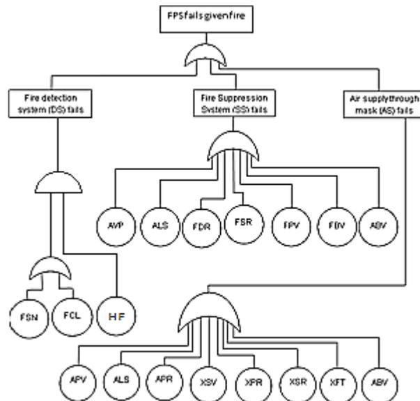
Figure 3 Fault Tree Model for FPS
