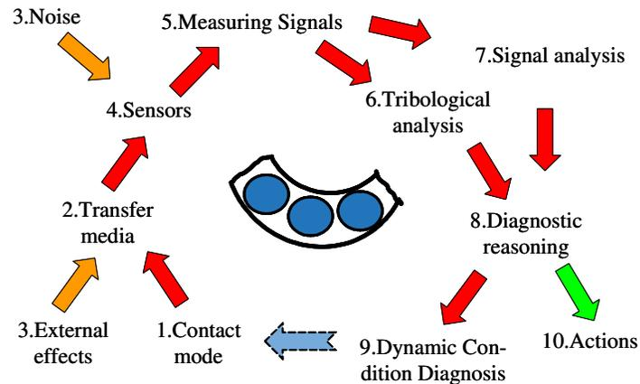
**Fig. 7:** The VTT Tribo-Diagnostic Circle Shows the Components and Path to Proceed from Contact Analysis over Monitoring, Signal Analysis and Diagnostics to Prognostics and Maintenance Decisions
