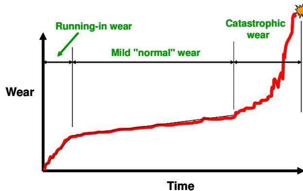
**Fig. 4:** The Wear Process Proceeds with Three Typical Stages, the Running-in Wear, the Mild or "Normal" Wear and Catastrophic Wear Resulting to Failure
