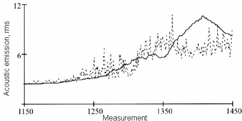
**Fig. 5:** Prognosis (Solid Line) Corresponding to a Time 3% in Future, Based on Measured Acoustic Emission rms-values (Dotted Line). This Means that e.g. the Prognosis for Measurement Point 1450 is Done Based on Measurement Data from 0 to 1407 [30]
