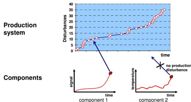
**Fig. 2:** Trends in the Physical Behaviour and Performance of Single Components are Monitored in the Component Level Approach while the Cumulative Number of Disturbances and Failure Events is Studied and Analysed in the System Level Approach. Figure adapted from [7].
