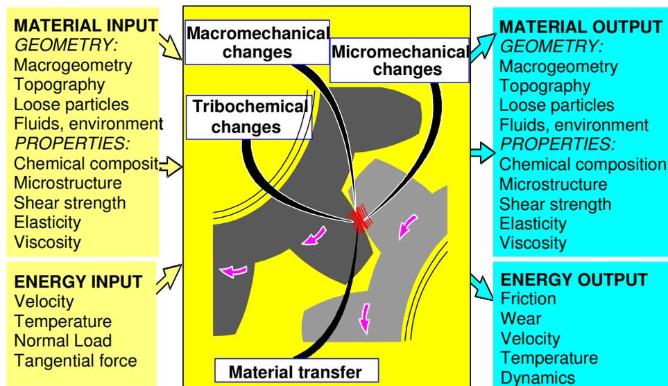
**Fig. 3:** The Tribological Process in a Contact Between Two Interacting Surfaces in Relative Motion Includes Mechanical and Chemical Changes that Depend on the Input Parameters and Result in Changed Contact Conditions and Changes the Output Parameters After a Certain Time
